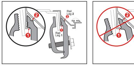
**Water Intrusion:** Make sure front retaining clamps are tight and properly engaged to the side rails. Check that the bulkhead seal is in place and the cover is resting on it. Make sure that all latches are engaged to the side rails and adjust if needed. Check that the side rails are installed flush with the top of the bed rail.
