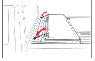
**FLIPPED UP POSITION:** Fold the cover (A) open and lift it until it's vertical towards your truck cab. Then release the prop rod that is attached to the side rail and clip it onto the ball stud on the underside of the cover.
