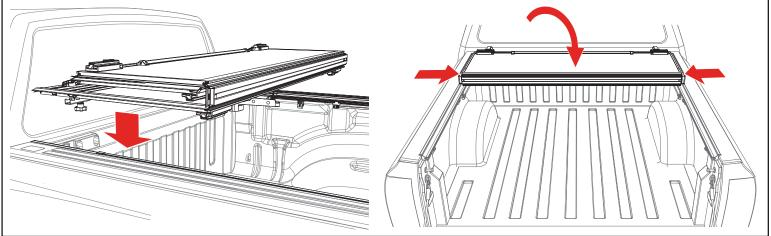
10 Rotate the cover retainer clamp (I) installed earlier so that it is aligned with its long side going side to side with the truck. The tabs of the cover retainer clamp (I) will align with the diagonal arm of the bed brace as shown. Align the retainer clamps on both sides and tighten the knobs by turning them clockwise until the lock washer is secure.
